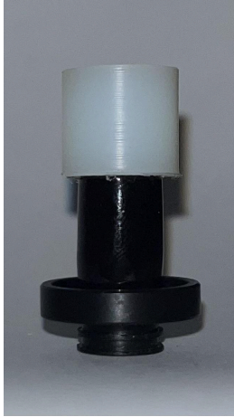
Figure 8: Optode with attachment cannot pass through the inner hole of the original mounting base (right).
