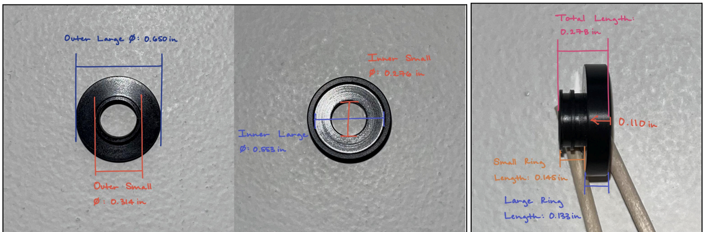
Figure 5: Dimensions of the back (left) and front (middle) profiles of the mounting base. Side profile (right) of the mounting base and dimensions.
