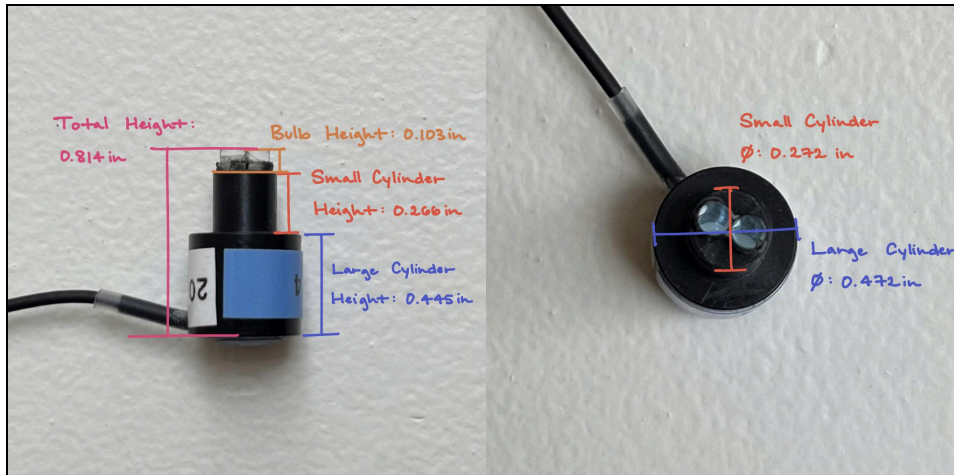
Figure 4: Side profile and dimensions of the detecting optodes.
