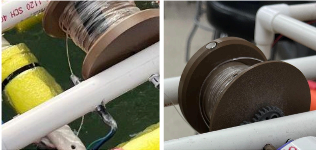
Figure 6a (left): The waterproofed Hall effect sensor is oriented perpendicular to the magnets and sits a distance of 0.5cm from the spool.
